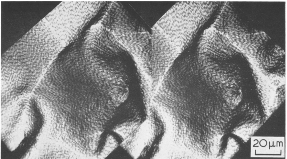
Figure 1 Stereo pair of a spherulite of polyethylene after radiation damage in the electron microscope, 6^\circ tilt between the pair.
